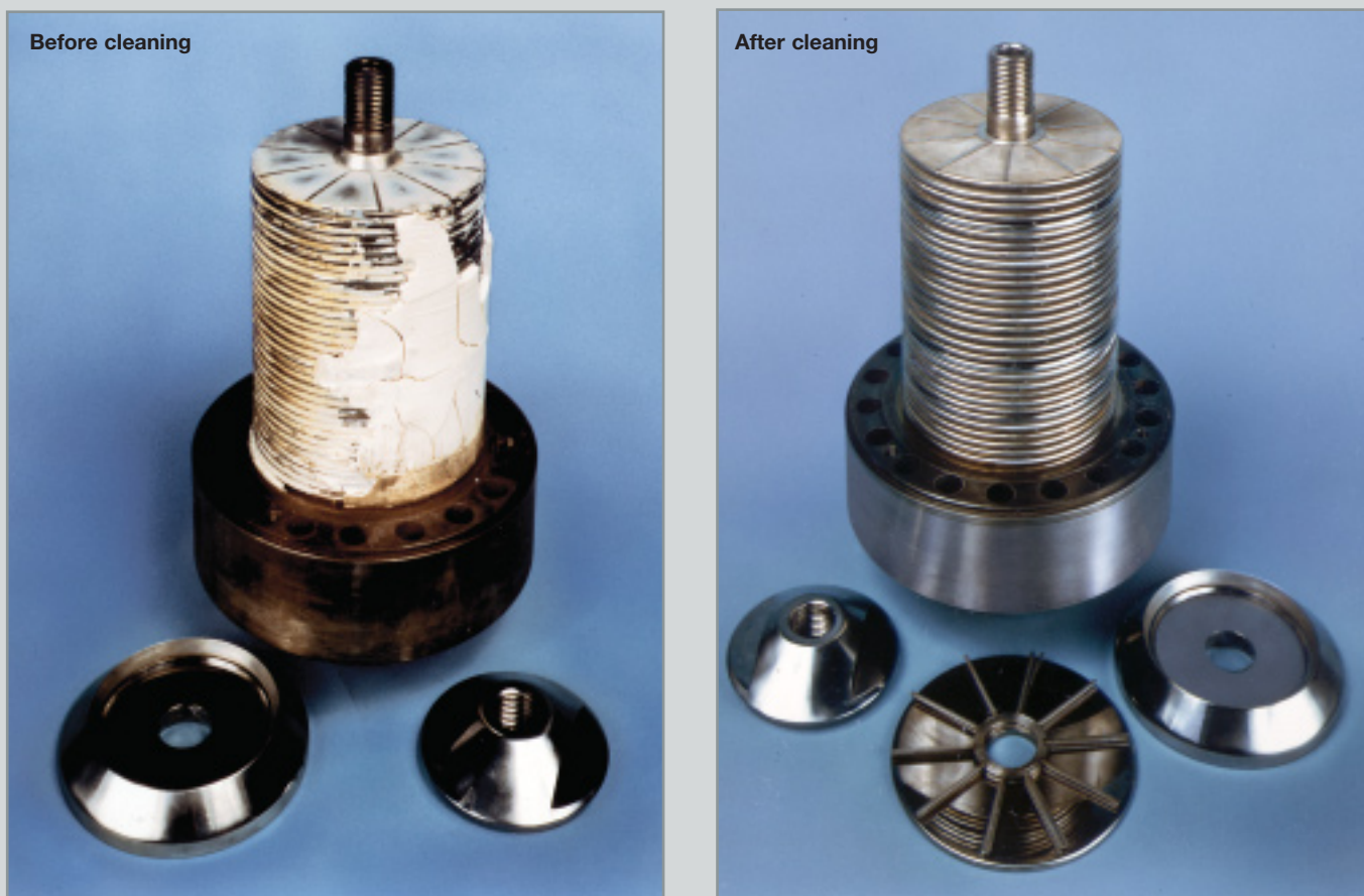
Figure 12 - Multi-segment stack assembly
