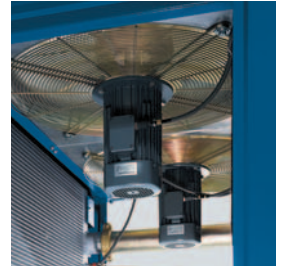
Plant cooling fan. The cool air passing through the unit picks up all radiant heat
