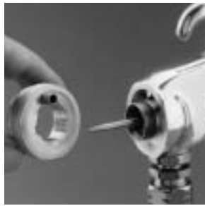
A REMOVEABLE AIR CAP BAFFLE EXTENDS THE GUN BODY SERVICE LIFE
